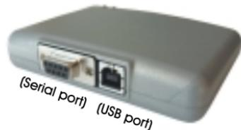
After the hardware has been connected for the first time, the blue LED will start flashing to show that the programmer is connected to the PC, but the driver has not yet been installed or loaded.
