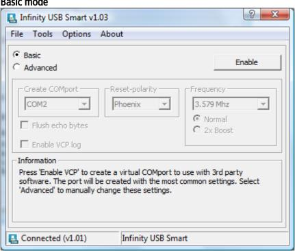
To control which com port is created or to change any of the default settings, select 'Advanced' mode and select the desired com port to create, and then press 'Enable'.
