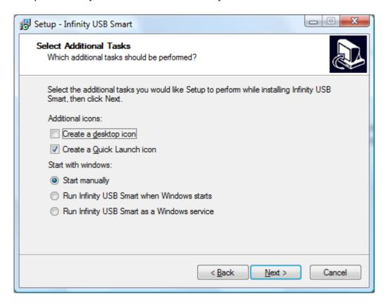
**Start manually:** This way you will have to start the Infinity USB Smart application manually, and enable the virtual comport with the settings you specify.
