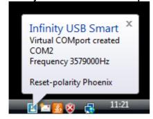
**Installing a module:** To add new custom features not available in the default Infinity USB Smart software a custom firmware module can be installed in the device, letting the device enumerate as a new USB device. Installing a module is **not** a firmware-upgrade of the Infinity USB Smart, it is a completely new device which is only activated by the physical switch.
