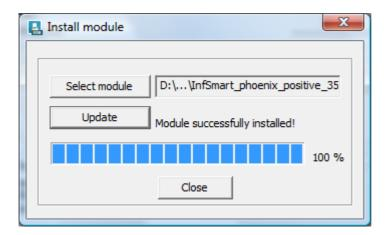
Select the correct module (.hex file) and press 'Update', the module will install in a few seconds. Once it is installed is can be activated by switching the bottom switch to the left position.
