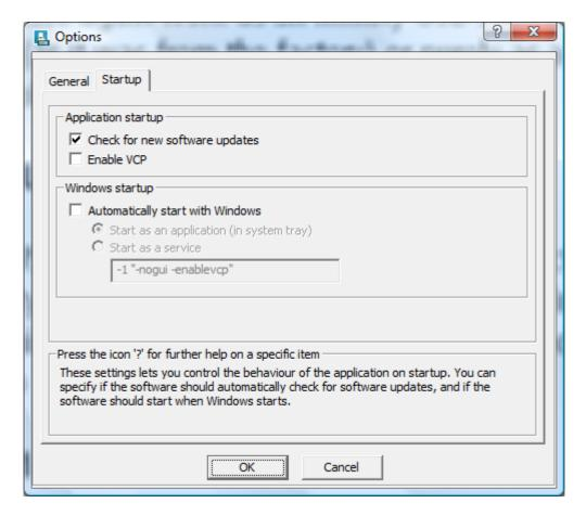
Default the software has to be started manually, the easiest way to start the software with Windows is to select "Automatically start with Windows" and then "Start as an application". This will launch the software and create the COM port when Windows starts, the software will be available as usual in the system tray.
